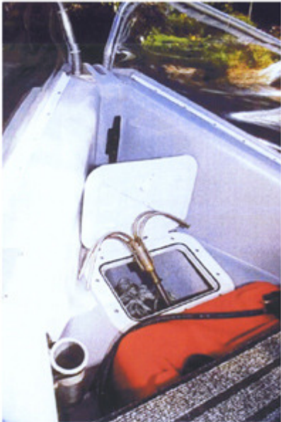
The anchor well is under a hatch in the forward platform. Bowrails contain the warp in the fairlead. Note tank under seat and forward rod storage holder.
